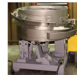
CCW Custom Airless Screw Feeder 21" Dia. #8x.625 Headed Blank at 600 + PPM w/out using air
