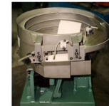
CW Custom Straight Parallel Screw Feeder 15" Dia. For Feeding Head Heavy Blanks on EW Menns
