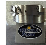
CCW Std Screw Feeder 18" Dia. Blanks from 3/16" — 2-1/2"
