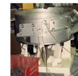
CW Outside Tooled Vibratory Screw Feeder 30" Dia. Blank Size #10 to 5/8 Popular w/ #20 & #30 Rollers
