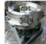
CCW Std Screw Feeder 15" Dia. Blanks from 3/16" — 1-1/2"
